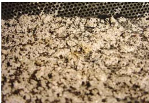
*Asbestos sprayed insulation unintentionally sprayed into a supply air duct during construction.*
